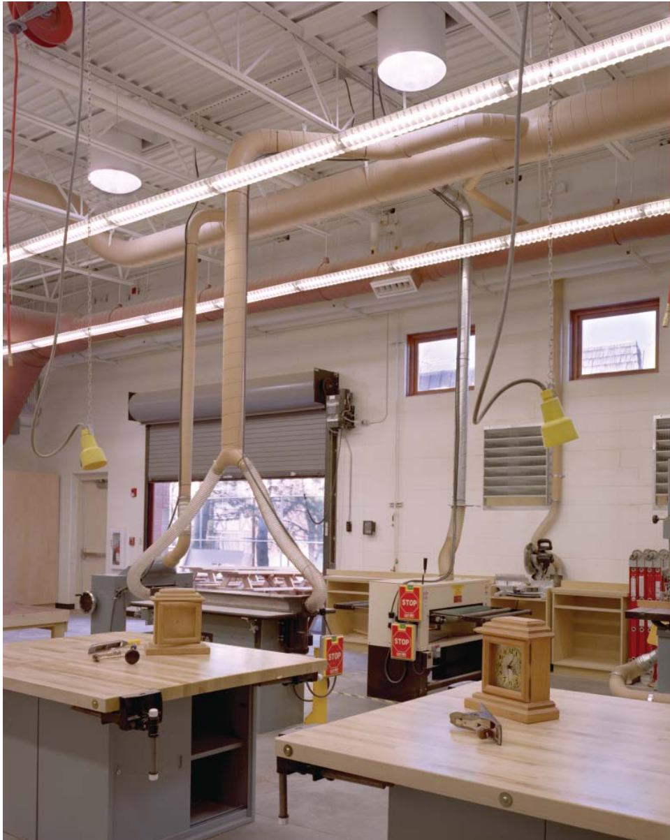
New Trades Workshop with Solar Tubes and Garage Door Providing Outdoor Connections and Daylighting Opportunities
